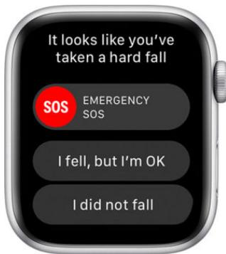
If the wearer is "immobile for about a minute," it begins a 15-second countdown. After that, the Watch will contact emergency services, which often can use mobile phone data to locate the wearer. Apple warns that it can't detect all falls.
